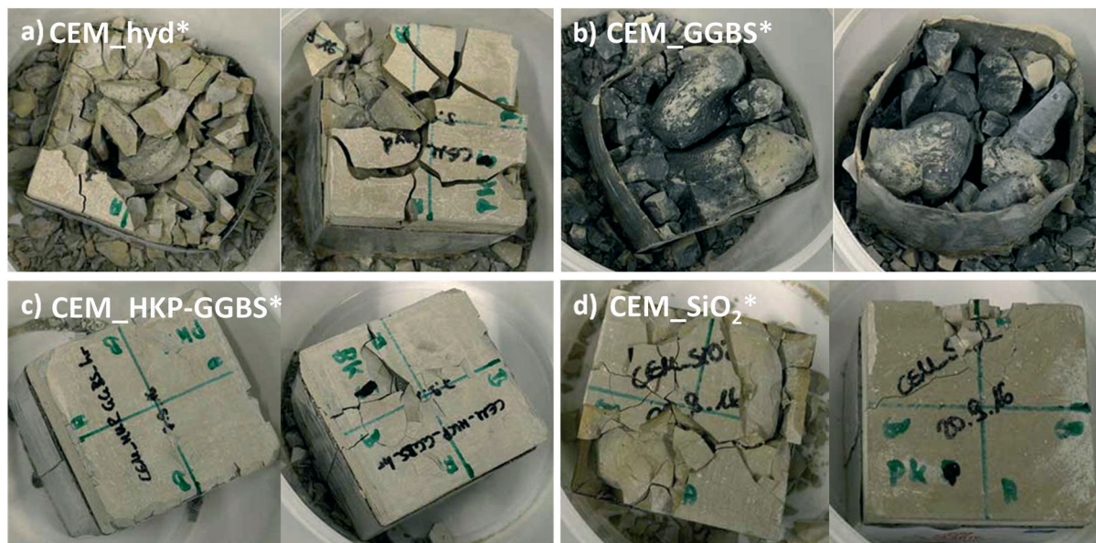
Fig. 1 Test specimens of a) CEM_hyd*, b) CEM_GGBS*, c) CEM_HKP-GGBS* and d) CEM_SiO 2 * after artificial freeze–thaw weathering.
