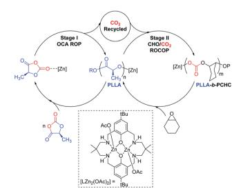
Scheme 1 Proposed polymerisation pathway whereby the di-zinc catalyst bridges two catalytic cycles: LLAOCA ROP and CO $_2$ /CHO ROCOP. Where [Zn] represents [LZn $_2$ (OAc) $_2$ ] during catalysis; R = initiating group and P = growing polymer chain.
