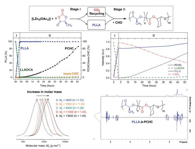
Fig. 1 The conversion vs. time data, determined from in situ <sup>1</sup>H NMR spectroscopy, during formation of PLLA-b-PCHC (top left). The changes in absorption intensity vs. time for selected resonances, from in situ IR spectroscopy (top right). Overlaid GPC analyses for isolated PLLA-b-PCHC samples (bottom left). The DOSY NMR spectrum of PLLA-b-PCHC (bottom right). Note: the structure of trans-CHC is illustrated in Fig. S23 (ESI†).
