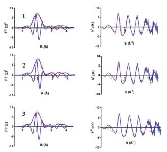
Fig. 4 Ir  $L_3$  edge EXAFS spectra of the Ir-pyalk WOC in solution (blue) comparing three simulated fit models from Fig. 3 (red dashed): mono- $\mu^2$ -oxo dimer **1**, bis- $\mu^2$ -oxo dimer **2**, and bis- $\mu^3$ -oxo cubane **3**. Displaying  $k^3$  weighted Fourier Transform (with imaginary part, left) and  $k^3$  weighted EXAFS plot (right) for each structure.
