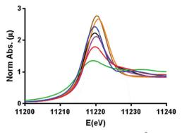
Fig. 1 Normalized XANES spectra calibrated to the Pt<sup>0</sup>  $L_3$  edge, displaying iridium  $L_3$  edge energies in  $Ir^0$  foil (green),  $[Ir^I(cod)Cl]_2$  (red),  $[Cp*Ir^{III}(H_2O)_3]SO_4$  (purple),  $[Cp*Ir^{III}(pyalk)Cl]$  (black),  $Na_2[Ir^{IV}Cl_6]$  (blue),  $Ir^{IV}O_2$  (orange), and the Ir-pyalk WOC (brown). For further details see Fig. S5 (ESI†).
