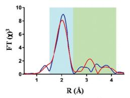
Fig. 2 Comparison of Ir  $L_3$  edge EXAFS data with  $k^3$ -weighting, showing Fourier transform EXAFS data for IrO<sub>2</sub> (red) and the Ir-pyalk WOC (blue).
