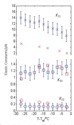
Fig. 5 The splay,  $K_{11}$  (crosses), twist,  $K_{22}$  (circles) and bend,  $K_{33}$  (squares) elastic constants as a function of  $T-T_{\rm NI}$  for compound 1. The experimental data are represented by the blue data points and the calculated data by the red data points. Note the break in the axis and the change in scale to make visible the very low twist and bend elastic constants.
