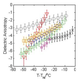
Fig. 8 Dielectric anisotropy,  $\Delta \varepsilon$  as a function of  $T - T_{NI}$  for compound 1 (black crosses), compound 2 (grey circles), mixture 1 (red downward triangles), mixture 2 (green upward triangles), mixture 3 (blue diamonds), mixture 4 (orange squares) and mixture 5 (magenta stars).
