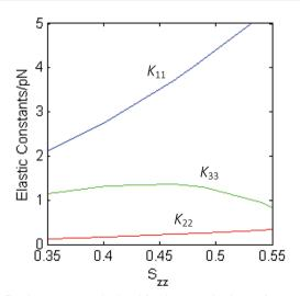
Fig. 7 Elastic constants calculated for the nematic phase of compound  ${\bf 1}$  as a function of the orientational order parameter  $S_{zz}$ , which quantifies the alignment of the z molecular axis (see Fig. 3) to the nematic director.
