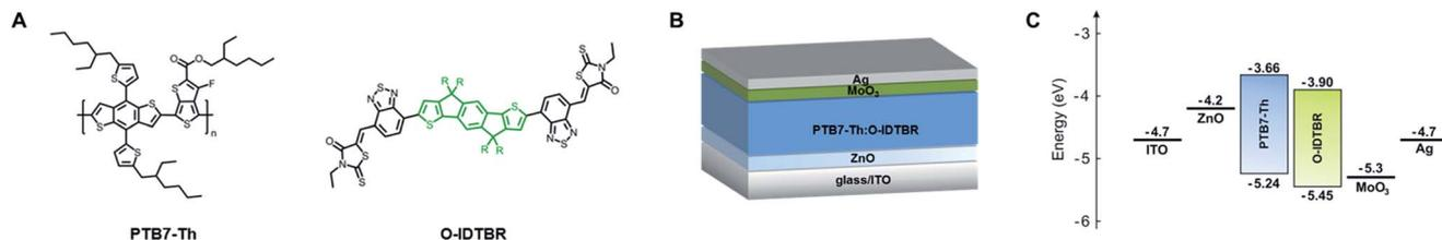
Fig. 1 (A) Chemical structures of PTB7-Th and O-IDTBR ( $R = n$ -octyl). The fused five-ring indaceno[1,2-*b*:5,6-*b'*]dithiophene core is highlighted in green. (B) Schematic representation of the examined bulk-heterojunction-type PTB7-Th:O-IDTBR solar cell in inverted architecture and (C) the corresponding energy level diagram related to the vacuum level. The energy levels of PTB7-Th and O-IDTBR were adopted from the literature.<sup>25,37</sup>
