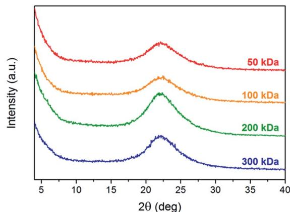
Fig. 4 Grazing incidence X-ray diffraction patterns of PTB7-Th thin films with different molecular weights (Cu  $K\alpha$  radiation,  $\lambda = 1.5406 \text{ \AA}$ ) deposited on silicon substrates by spin coating from *ortho*-dichlorobenzene solutions (normalized to layer thickness).
