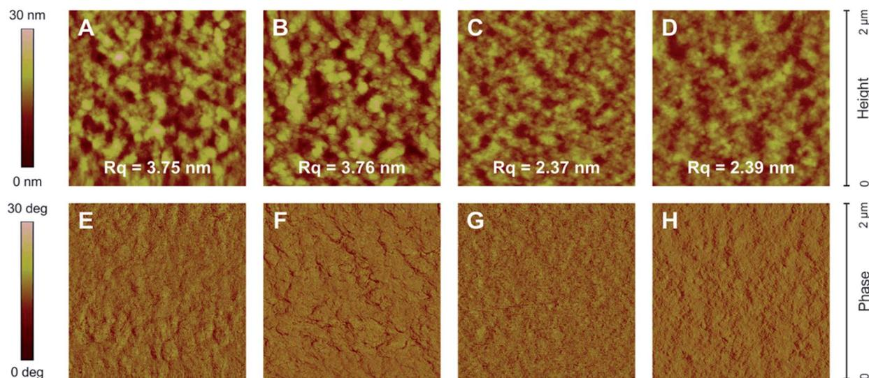
Fig. 5 AFM topography images (A–D) and phase images (E–H) of PTB7-Th:O-IDTBR blend thin films with a molecular weight of 50 kDa (A and E), 100 kDa (B and F), 200 kDa (C and G), and 300 kDa (D and H) of PTB7-Th (image size:  $2 \times 2 \mu\text{m}$ ).
