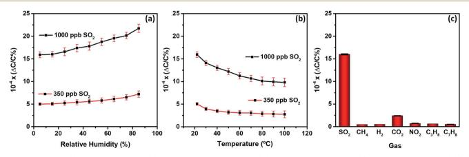
Fig. 4 Effects of the (a) relative humidity and (b) temperature on the MFM-300 (In) MOF sensor performance. (c) Selectivity of the MFM-300 (In) MOF sensor to other gases at 1000 ppb.
