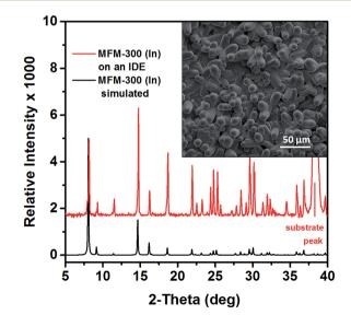
Fig. 2 Comparison of calculated X-ray diffraction (XRD) patterns of MFM-300-MOF (In) and thin film grown on the IDE. Top view SEM image of MFM-300-MOF (In) coating.
