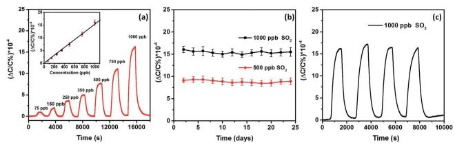
Fig. 3 (a) Detection of  $SO_2$  in the 75 to 1000 ppb concentration range, insets: linear response for the corresponding range; (b) linear response for MFM-300 (In) MOF-based sensor upon exposure to 500 and 1000 ppb of  $SO_2$  over a 24 day period; (c) reproducibility cycles for the detection of 1000 ppb of  $SO_2$ .
