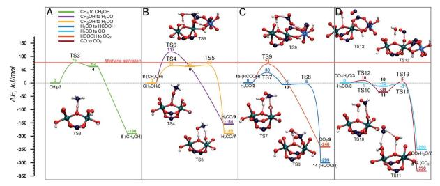
Fig. 4 Energy diagram of cycle I, schematic representation is shown in Fig. 2. (A)  $CH_4 \rightarrow CH_3OH$ , (B)  $CH_3OH \rightarrow CH_2O$  in two steps (yellow) and in one step (purple), (C) H<sub>2</sub>CO → HCOOH (dark blue), and its consecutive oxidation to CO<sub>2</sub> (orange), (D) CH<sub>2</sub>O → CO (light blue) and its consecutive oxidation to CO<sub>2</sub> (brown). The reference point for all reactions is the active site and the adsorbed molecule as represented in Fig. 2.
