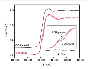
Fig. 3 Comparison of operando XANES spectra recorded at Mo K-edge for a 2MoHZ-13 catalyst during consecutive pulsing of CH<sub>4</sub> at 700 °C (pink curves) and a 2MoHZ-13 catalyst carburized at 780 °C with a 30 ml min<sup>-1</sup> flow of 2.5% CO in He (black curve).
