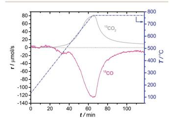
Fig. 1  $^{13}$ CO consumption and simultaneous  $^{13}$ CO $_2$  production in TPC of 2MoHZ-13 with 30 ml min $^{-1}$ , 2.5%  $^{13}$ CO in He. The temperature was increased to 780  $^{\circ}$ C at a rate of 10  $^{\circ}$ C min $^{-1}$  (right axis). (*cf.* Fig. S4† for TPC for all Mo loadings).
