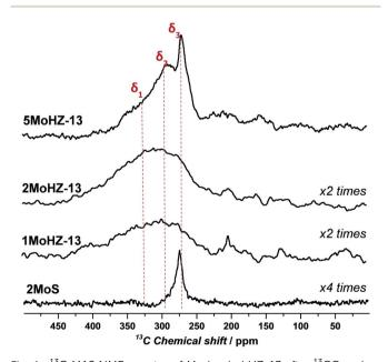
Fig. 4  $^{13}$ C MAS NMR spectra of Mo loaded HZ-13 after  $^{13}$ CO carburization at 780  $^{\circ}$ C for 1 h using 30 ml min $^{-1}$ , 2.5%  $^{13}$ CO in He. Deconvolution results of the spectra can be found in Fig. S18.†
