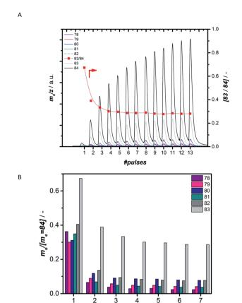
Fig. 5 Evolution of masses typical for the fragmentation of benzene at a consecutive pulsing of 223  $\mu$ mol  $^{13}$ CH<sub>4</sub> (Panel A) to the 300 mg 2MoHZ-13 catalyst carburized at 780 °C with 30 ml min<sup>-1</sup> 2.5%  $^{12}$ CO in He. Panel B shows the area under each pulse for masses 78 to 83 normalized by  $m_e=84$ .
