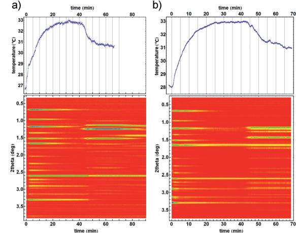
Fig. 2 Time resolved diffractograms with their temperature profiles for crystallisation of the (a) *kat* polymorph of ZIF-8 from the amorphous matrix and (b) crystallisation directly into the *dia* polymorph. Homogeneity and uniformity of the reaction mixture is evident from the uniformity of the diffraction signal from crystalline silicon (at 2.6° in 2theta) which was used as an internal scattering standard.<sup>22</sup>
