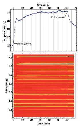
Fig. 5 Mechanochemical formation of a pillared MOF material. Starting from ZnO, terephthalic acid, and dabco (1,4-diazabicyclo [2.2.2]octane),<sup>50</sup> the formation of a fleeting short-lived intermediate (X-ray reflection at 0.5° in 2theta) around 4 minutes of milling can be observed in the temperature profile as an interruption in the heating profile.
