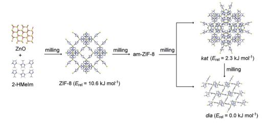
Fig. 1 Reaction sequence of mechanochemical crystallisation—amorphisation—recrystallisation of ZIF-8. Relative energies ( $E_{rel}$ ) of ZIF-8 and its polymorphs are taken from ref. 30.
