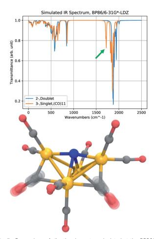
Fig. 7 Comparison of vibrational spectra calculated at the BP86/6-31G\*-LDZ level for  ${\bf 1}^{2-}$  (blue) and  ${\bf 2}^{3-}$  (orange). The IR spectrum of  ${\bf 2}^{3-}$  has a distinct peak red-shifted from the main band of CO-stretches by about 150 cm $^{-1}$  (green arrow), corresponding to a symmetric and antisymmetric stretch of the bridging CO ligands (bottom). An artificial Lorentzian broadening of 10 cm $^{-1}$  is used.
