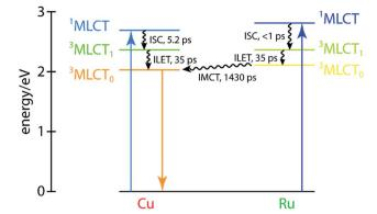
Fig. 8 Jablonski diagram for  $CuMe_2-RuH_2$  with the copper- and ruthenium-centered states shown on the left and right sides, respectively. The energies of both  $^1MLCT$  states and the coppercentered  $^3MLCT_0$  state are estimated from steady-state absorption and emission measurements, and all other energies are qualitative estimates.
