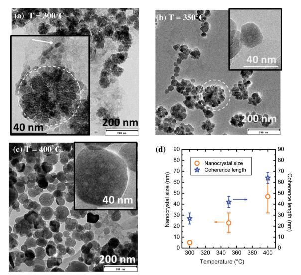
Fig. 4 (a–c) TEM images of YAG:Ce nanocrystals synthesized at different reaction temperatures with P = 200 bar, [Al] = 0.09 mol L<sup>-1</sup> and t = 150 min. In the inset of (a), the arrow points an individual nanocrystal and the dashed circle emphasizes an aggregate. (d) Evolution of the nanocrystal size (determined by TEM, orange circles, error bars corresponding to size dispersion) and coherence length (determined by PXRD, blue stars) as a function of reaction temperature.
