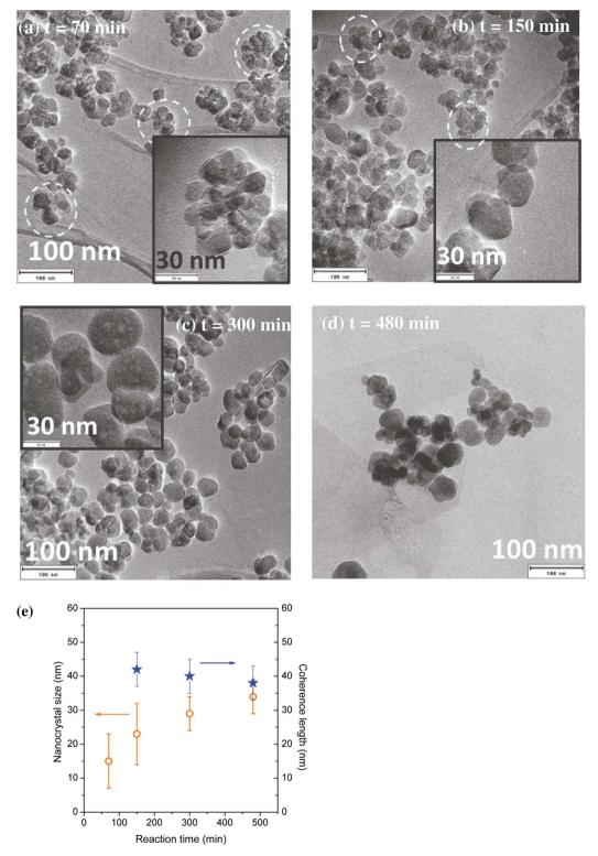
Fig. 6 (a-d) TEM images of YAG:Ce nanocrystals synthesized for different reaction times. P = 200 bar, T = 350 °C, [Al] = 0.09 M. (e) Evolution of the coherence length (blue stars) and the nanocrystal size (orange circles, error bars corresponding to size dispersion) as a function of the reaction time under these conditions.
