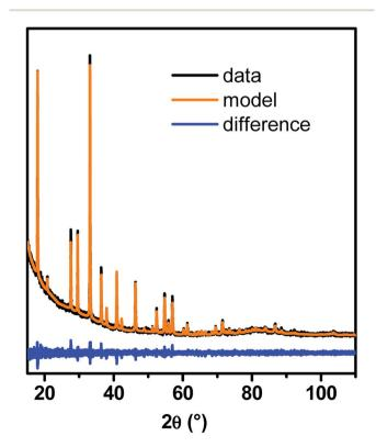
Fig. 1 Typical PXRD pattern of YAG:Ce nanocrystals synthesized with our modified solvothermal method and its corresponding Le Bail fit.
