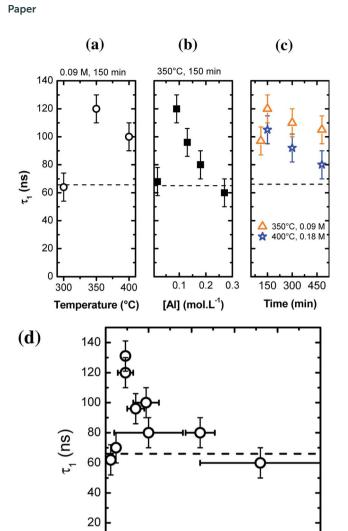
Fig. 9 (a–c) Excited state lifetime  $\tau_1$  of Ce<sup>3+</sup> as a function of various synthesis parameters, indicated on the graph (with P=200 bar). The dashed line represents the excited state lifetime of bulk YAG:Ce. (d) Evolution of  $\tau_1$  as a function of the particle size.
