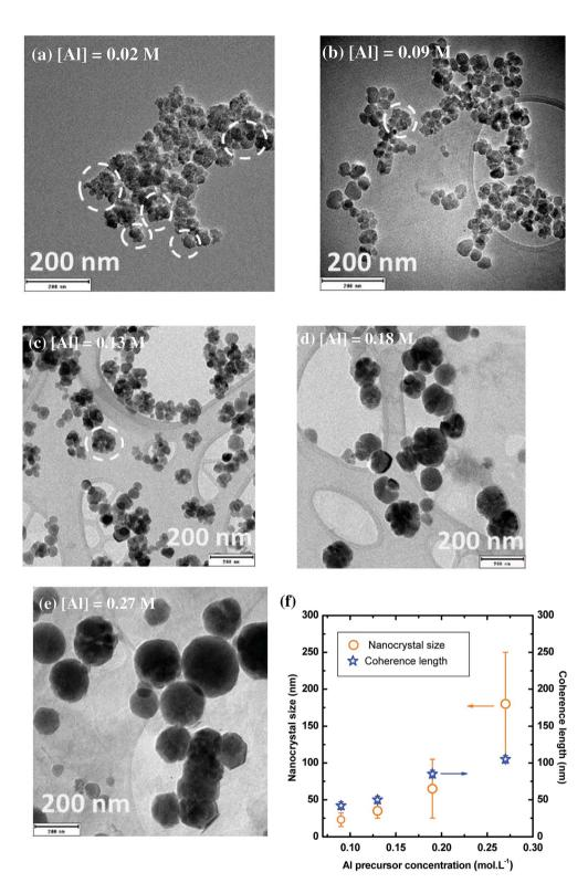
Fig. 5 (a–e) TEM images of YAG:Ce nanocrystals synthesized with different precursor concentrations. P=200 bar, T=350 °C and reaction time = 150 min. (f) Evolution of the nanocrystal size (orange circle, error bars corresponding to size dispersion) and coherence length (blue star) as a function of the precursor concentration. Coherence length larger than 100 nm cannot be measured to instrumental limitation.
