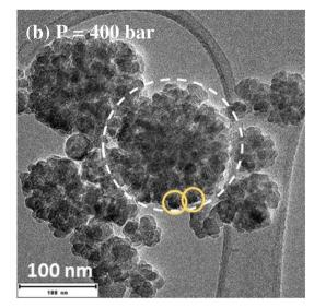
Fig. 3 TEM images of YAG:Ce nanocrystals synthesized at different pressure with T = 350 °C, [Al] = 0.09 mol L<sup>-1</sup> and reaction time = 150 min. Some individual nanocrystals are circled with yellow solid lines. An aggregate is circled with a white dashed line.
