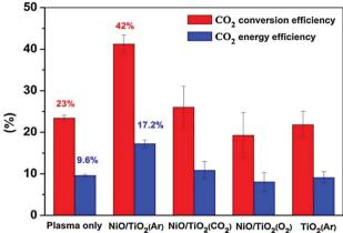
Fig. 5  $CO_2$  conversion and energy efficiencies, measured during the plasma-catalysis  $CO_2$  dissociation, are shown for the NiO/TiO<sub>2</sub> catalysts prepared by plasma treatment with different gases (O<sub>2</sub>, Ar, CO<sub>2</sub>). Reproduced from ref. 198 with permission from Elsevier, copyright 2016.
