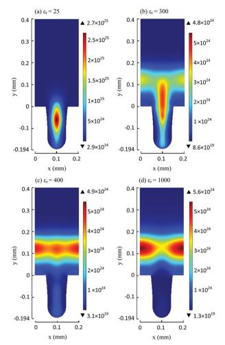
Fig. 8 Distributions of the electron impact ionization rate, averaged over time in one AC cycle, for different dielectric constants: (a)  $\epsilon_r=25$ , (b)  $\epsilon_r=300$ , (c)  $\epsilon_r=400$ , and (d)  $\epsilon_r=1000$ , for a helium discharge sustained at 20 kV with a 100  $\mu m$  pore. Reproduced from ref. 223 with permission from American Chemical Society, copyright 2016.
