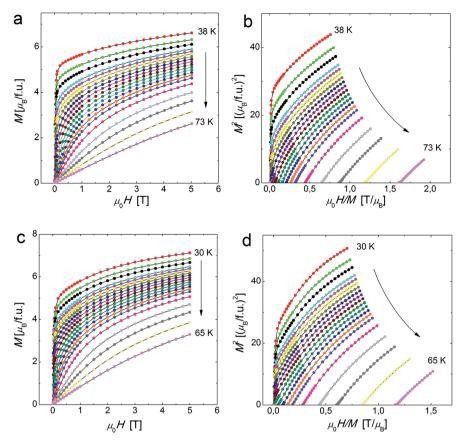
Fig. 3 Magnetization versus field isotherm measured at temperatures in the vicinity of  $T_c$  for MnNb (a) and FeNb (c). The Arrott plots ( $M^2$  vs. H/M) at the vicinity of  $T_c$  for MnNb (b) and FeNb (d).
