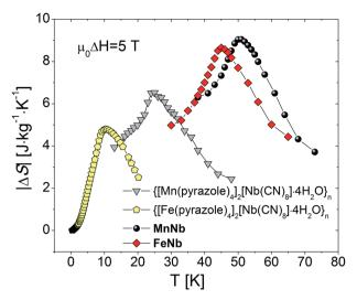
Fig. 5 Magnetic entropy change of MnNb, FeNb and  $\{[M^{II}(pyrazole)_4]_2[Nb^{IV}(CN)_8]\cdot 4H_2O\}_n$  (M = Mn, Fe) determined for magnetic field change from 0 to 5 T.
