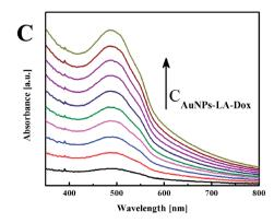
Fig. 3 (A) UV-Vis spectra of AuNPs-LA with increasing concentrations and (B) calibration curves for various wavelengths. (C) Spectra for increasing concentrations of AuNPs-LA-Dox.
