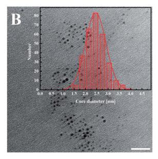
Fig. 1 TEM images of (A) AuNPs-LA and (B) AuNPs-LA/LAFA. The scale bar is 20 nm. The histograms show the size distributions of the AuNPs evaluated from the TEM images.
