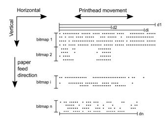
Fig. 5 To determine  $t_{\rm req}$  for any pattern, the pattern needs to be divided into n bitmaps. In the  $i^{\rm th}$  bitmap,  $d_i$  is the index of the rightmost droplet to dispense. The dimension of bitmap i then equals  $r \times d_i$ , where r is the number of nozzles for a particular color of the printer. To simplify the figure, r was chosen to be 4. The Epson Stylus SX235W actually has 90 black nozzles and 29 nozzles per color.
