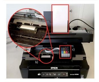
Fig. 3 The modified Epson Stylus SX235W with (a) lengthwise sliced plain paper, (b) a microscope glass slide placed over the piece of metal, whose height can be adjusted and (c) refillable cartridges to experiment with other fluids.
