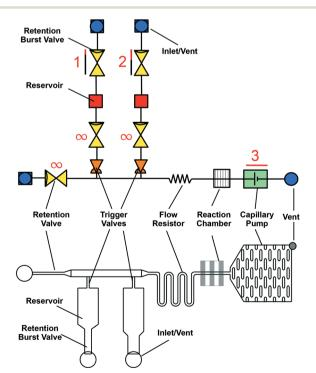
Fig. 5 Symbolic (top) and schematic (bottom) representations of a microfluidic circuit consisting of several capillary fluidic elements including: capillary pump, trigger valve, retention valve, retention burst valve, flow resistor, inlets, and vents. Fig. S1<sup>†</sup> provides an editable version of this image as well as symbolic representations of individual capillaric elements to enable others to re-use and edit our proposed symbols and highlight their own modular designs.
