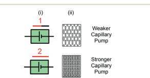
Fig. 6 (i) Symbolic and (ii) schematic representation of capillary pump. The spacing between microstructures in the pump determines its capillary pressure. Stronger capillary pumps have more closely spaced microstructures.
