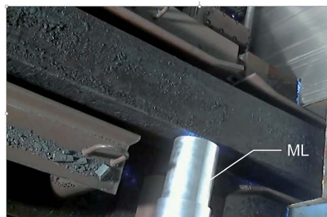
Fig. 7 Inline measurement of steel blooms, left: the bloom is transported on a roller table and arriving from the left, right: the measuring lance (ML) is approached to the side face of the bloom, laser irradiation is activated to locally ablate the scale layer and to analyse the bulk composition. Diameter of ML: 170 mm. 32
