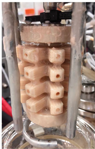
Fig. 2 3-D printed fermenter agitator with attached biofilm after 750 h continuous fermentation.
