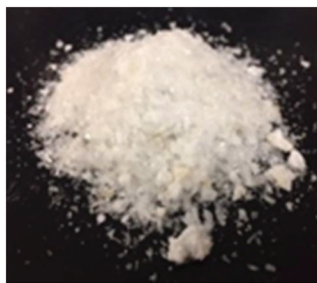
Fig. 8 Succinic acid crystals recovered from continuous fermentation broth of PAL.
