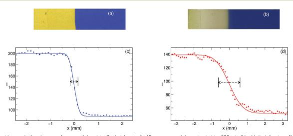
Fig. 2 Front images in the absence of nanoparticles at t = 7 min (a) and with 15 mg nanoparticle content at t = 230 min (b) with their front profiles (c and d) in gels of V = 8 cm<sup>3</sup>. The fitted cumulative normal distribution function is shown by solid lines and the appropriate front width is indicated with arrows. The length of the gel strips is 6.5 cm (a) and 5.8 cm (b)
