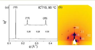
Fig. 2 (a) Powder SAXS curve of IC3/12 recorded at 80 °C at station I22 at Diamond. (b) GISAXS diffraction pattern of IC3/12 recorded at 80 °C on beamline B28 at ESRF.
