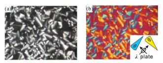
Fig. 1 Polarized optical microscopy textures of IC3/14 at 70 °C. (b) is recorded with a full-wave (λ) plate. For explanation of colours see ESI.†
