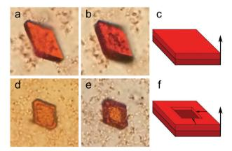
Fig. 1 Optical images of supercrystals appearing in a course of CdSe quantum dots self-assembling. Panels a, b, d, and e show optical images (20  $\times$  20  $\mu$ m) of typical SC<sub>4.0</sub> in transmitted white light captured after 12 (a) and 31 (b) days for a layered supercrystal nucleation, and after 3 (d) and 5 (e) days for partly layered supercrystal nucleation. Panels c and f show layered and partly layered supercrystal nucleations, respectively
