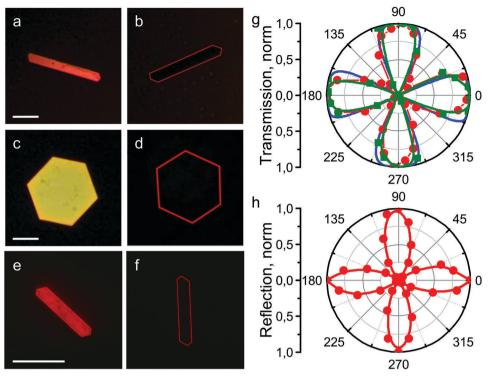
Fig. 5 Microphotographs of the supercrystals  $SC_{4.0}$  (a, b, e and f) and  $SC_{3.1}$  (c and d) recorded with  $20 \times$  objective (NA = 0.75) under transmitted (a–d) and reflected (e and f) light respectively. Scale bars are  $20 \mu m$ . Angular dependences of transmitted (g) and reflected (h) light between crossed polarizers for  $SC_{4.0}$  (red curves),  $SC_{3.1}$  (green curve), and the organic matrix (blue curve).
