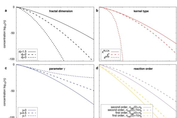
Fig. 8 Effect of different kernel types and parameters on the modelled particle size distribution. (a) Effect of the aggregate fractal dimension (kernel used k<sup>c</sup>). (b) Comparison of kernel types—reaction limited cluster aggregation kernel, constant kernel, simple polymerisation kernel. (c) Effect of parameter  $\gamma$  in a RLCA kernel. (d) Binary aggregation versus aggregation via a unimolecular process from eqn (8)
