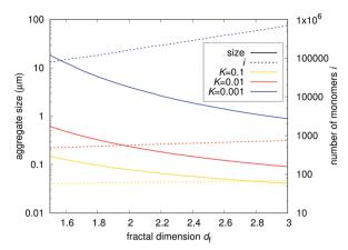
Fig. 9 Estimated maximum sizes of fractal aggregates in a typical biopharmaceutical sample. The solid lines represent the physical size of aggregates in  $\mu$ m. The dashed lines represent the number of primary particles comprising the aggregates. The results for different ratios between unimolecular and subsequent bimolecular process rates K are shown. The fractal nature of the aggregates has a significant impact on aggregation dynamics.
