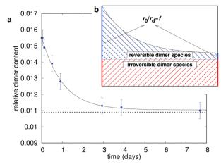
Fig. 6 Experimental determination of mAb 3 dimer reversibility. (a) Dimer/ monomer concentration and a fit of eqn (18) - solid line. The dotted line corresponds to the estimated irreversible dimer content. (b) A schematic interpretation of monomer/dimer dynamics after dilution. If the ratio r after dilution remains much higher than 1/f of the starting ratio when equilibrium is achieved, an irreversible dimer species is most likely present in the sample
