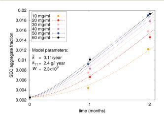
Fig. 5 Experimental characterisation of unimolecular aggregation of mAb 2. Relative SEC aggregate content measurements are overlaid with a fitted model (dotted lines), with the model parameters displayed. The model assumes a purely unimolecular first aggregation step.
