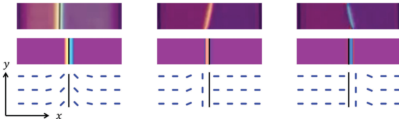
Fig. 15 Calculated images of polarizing micrographs (polarizer and analyzer along x and y and diagonal \lambda plate) for the model director field near symmetric and asymmetric twist disclinations, confined to a narrow region around the disclination line, as described in the text. Top row: Experimental micrographs (same as in Fig. 4). Middle row: Calculated micrographs, the black line indicates the position of the disclination line. Bottom row: Schematics of the director field in the plane containing the disclination line (black line, note that the lateral scale of the schematics is not the same as in the micrographs but \approx 10 times expanded). Left panel: Symmetric configuration of the twist disclination ( \varphi_0 = \frac{\pi}{2} ). Middle and right panel: the two asymmetric configurations ( \varphi_0 = 0 and \frac{\pi}{2} ).
