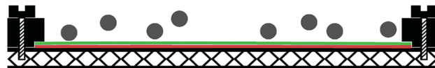
Fig. 5 Cross section of the vessel. The crossed shaded area represents the bottom plate made from aluminium honeycomb material, the black area marks the frame made from Perspex. The green (red) line represents the glass plate (the electroluminescence sheet), respectively.
