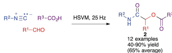
Scheme 2 The mechanochemical Passerini reaction.
