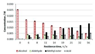
Fig. 2 Reaction profile obtained at different residence times. Conditions: oxidation of benzyl alcohol (feed 1 = 50 mM in methanol) with  $H_2O_2$  (feed 2 = 100 mM in  $H_2O_2$ ) over Au/TiO<sub>2</sub> at 70 °C, flow rates  $= 0.05-1 \text{ mL min}^{-1}$
