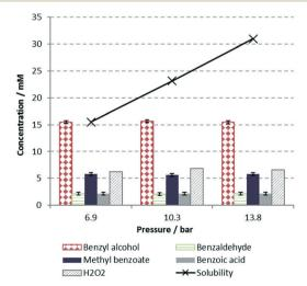
Fig. 3 Effect of pressure on reaction outcome, plotted with the estimated solubility of O2, as predicted by Henry's law, using the Ostwald's coefficient reported by Tokunaga. 4b Conditions: benzyl alcohol in MeOH/H<sub>2</sub>O (25 mM), 2 equiv. of H<sub>2</sub>O<sub>2</sub>, 70 °C, 200 mg Au/  $TiO_2$ ,  $\tau = 13$  seconds.
