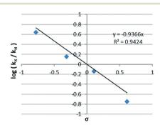
Fig. 4 Hammett plot for the aldehyde formation step, where  $k_X$  and  $k_{\rm H}$  are the  $k_{\rm 1}$  rate constants for the para-substituted (X = Me, MeO, Cl,  $CF_3$ ) and unsubstituted (X = H) benzyl alcohols, respectively. Reaction conditions: 25 mM alcohol in MeOH/H<sub>2</sub>O, 2 equivalents of H<sub>2</sub>O<sub>2</sub>, 100 mg Au/TiO2, 200 psi, 70 °C
