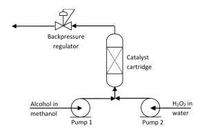
Fig. 5. General schematic of the flow reactor used in the kinetic
