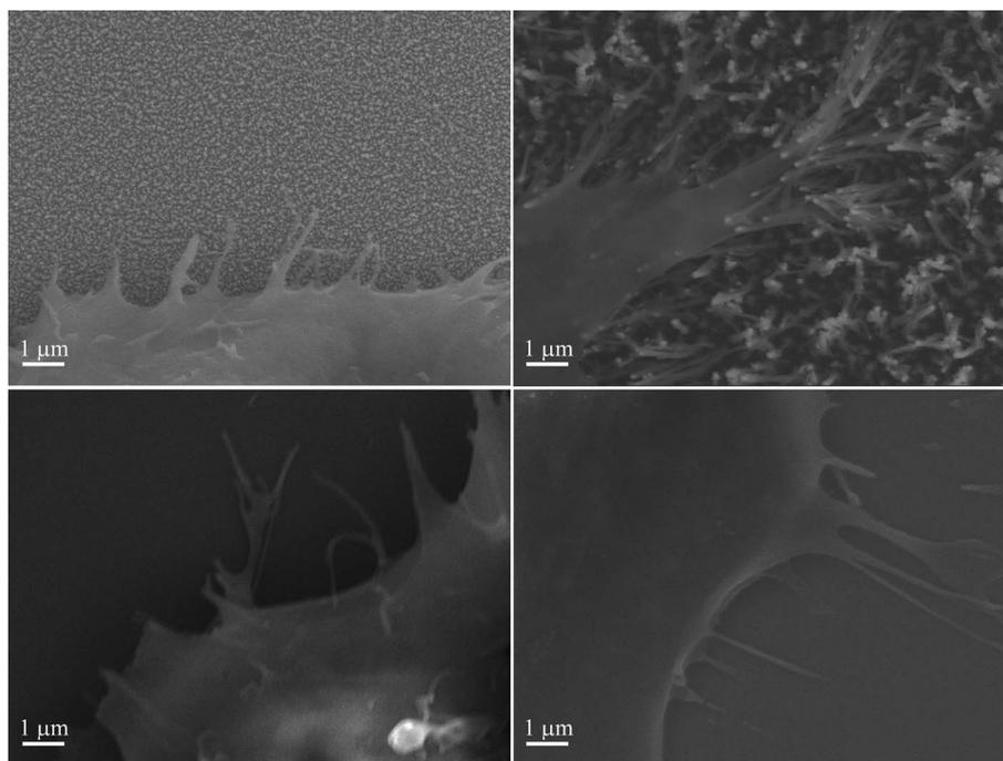
Fig. 6 mNSC on (A) Pt-CNFs, (B) Ni-CNFs, (C) Pt thin film, and (D) ta-C. Extensive amount of filopodia is observed on Ni-CNFs compared to other tested materials.
