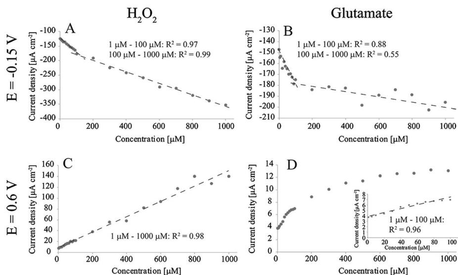
**Fig. 2** Amperometric detection of H<sub>2</sub>O<sub>2</sub> and glutamate in non-degassed PBS with Pt-CNFs. (A) H<sub>2</sub>O<sub>2</sub> at E = −0.15 V vs. Ag/AgCl. (B) Glutamate at E = −0.15 V vs. Ag/AgCl. (C) H<sub>2</sub>O<sub>2</sub> at E = 0.6 V vs. Ag/AgCl. (D) Glutamate at E = 0.6 V vs. Ag/AgCl.
