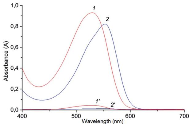
Fig. 5 Absorption spectra of the ion association pair in organic phase:  $2.2 \times 10^{-6}$  mol L<sup>-1</sup> Cr(vi);  $3.0 \times 10^{-4}$  mol L<sup>-1</sup> KI;  $1.6 \times 10^{-4}$  mol L<sup>-1</sup> ABR; 0.2 mol L<sup>-1</sup> H<sub>2</sub>SO<sub>4</sub>; 250 μL organic phase; vortexing 15 s, 3000 rpm; centrifugation 2 min, 1500 rpm; 1 – isoamylacetate; 2 – benzene; 1', 2' – respectively blank tests.
