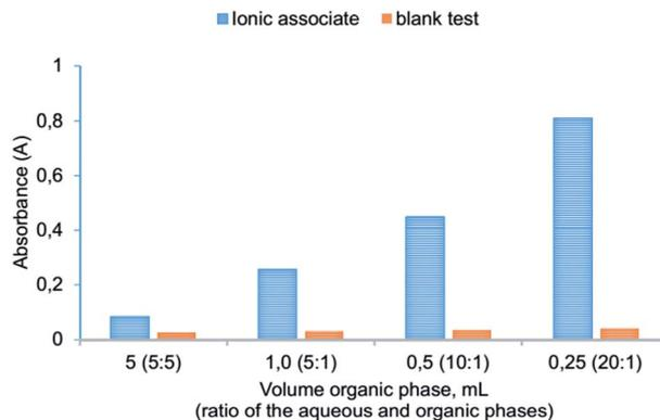
Fig. 7 Effect of the ratio of the aqueous and organic phases on the absorbance:  $2.0 \times 10^{-6}$  mol L<sup>-1</sup> Cr(vi);  $3.0 \times 10^{-4}$  mol L<sup>-1</sup> KI;  $1.6 \times 10^{-4}$  mol L<sup>-1</sup> ABR; 0.2 mol L<sup>-1</sup> H<sub>2</sub>SO<sub>4</sub>; volume aqueous phases 5.0 mL; vortexing 15 s, 3000 rpm; centrifugation 2 min, 1500 rpm.
