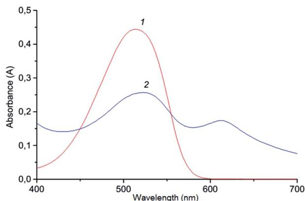
Fig. 1 Absorption spectra of the ABR (1) and ion association pair ABR with  $\text{I}_3^-$  (2) in aqueous solution: 1– $2.3 \times 10^{-5} \text{ mol L}^{-1}$  ABR;  $0.2 \text{ mol L}^{-1} \text{ H}_2\text{SO}_4$ ; 2– $2.3 \times 10^{-5} \text{ mol L}^{-1}$  ABR;  $1.3 \times 10^{-5} \text{ mol L}^{-1}$  Cr(vi);  $3.0 \times 10^{-4} \text{ mol L}^{-1}$  KI;  $0.2 \text{ mol L}^{-1} \text{ H}_2\text{SO}_4$ .
