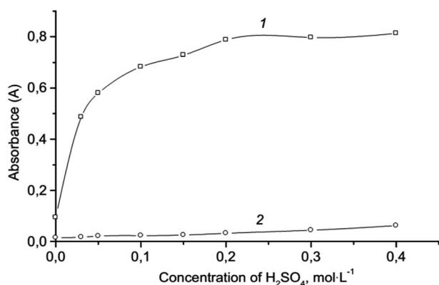
Fig. 2 Effect of the H<sub>2</sub>SO<sub>4</sub> concentration on the microextraction:  $2.0 \times 10^{-6}$  mol L<sup>-1</sup> Cr(vi);  $3.0 \times 10^{-4}$  mol L<sup>-1</sup> KI;  $1.6 \times 10^{-4}$  mol L<sup>-1</sup> ABR; 250  $\mu$ L isoamylacetate; vortexing 15 s, 3000 rpm; centrifugation 2 min, 1500 rpm; 1 – ion associate; 2 – blank test.
