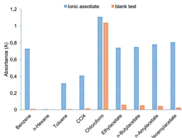
Fig. 4 Extraction efficiency using different solvents:  $2.0 \times 10^{-6}$  mol L<sup>-1</sup> Cr(vi);  $3.0 \times 10^{-4}$  mol L<sup>-1</sup> KI;  $1.6 \times 10^{-4}$  mol L<sup>-1</sup> ABR; 0.2 mol L<sup>-1</sup> H<sub>2</sub>SO<sub>4</sub>; 250  $\mu$ L organic solvents; vortexing 15 s, 3000 rpm; centrifugation 2 min, 1500 rpm.
