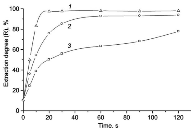
Fig. 6 Effect of techniques microextraction on the extraction efficiency:  $2.0 \times 10^{-6}$  mol L<sup>-1</sup> Cr(vi);  $3.0 \times 10^{-4}$  mol L<sup>-1</sup> KI;  $1.6 \times 10^{-4}$  mol L<sup>-1</sup> ABR; 0.2 mol L<sup>-1</sup> H<sub>2</sub>SO<sub>4</sub>; 250 μL isoamylacetate; 1 – vortex mixer (3000 rpm); 2 – magnetic stirrer (1200 rpm); 3 – manual shaking (100 shaking in a minute).
