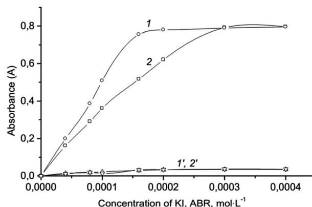
Fig. 3 Effect of the ABR (1) and KI (2) concentration on the absorbance of ionic associate extracts:  $2.0 \times 10^{-6}$  mol L<sup>-1</sup> Cr(vi); 0.2 mol L<sup>-1</sup> H<sub>2</sub>SO<sub>4</sub>; 250  $\mu$ L isoamylacetate; vortexing 15 s, 3000 rpm; centrifugation 2 min, 1500 rpm; 1– $3.0 \times 10^{-4}$  mol L<sup>-1</sup> KI; 2– $1.6 \times 10^{-4}$  mol L<sup>-1</sup> ABR; 1', 2' – respectively blank tests.
