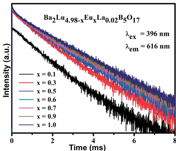
Fig. 5 PL decay curves of  $\text{Ba}_2\text{Lu}_{4.98-x}\text{Eu}_x\text{La}_{0.02}\text{B}_5\text{O}_{17}$  ( $x = 0.1, 0.3, 0.5, 0.6, 0.7, 0.9$  and  $1.0$ ) under excited at 396 nm and monitored at 616 nm.
