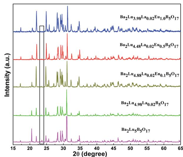
Fig. 1 XRD profiles of the  $\text{Ba}_2\text{Lu}_5\text{B}_5\text{O}_{17}$ ,  $\text{Ba}_2\text{Lu}_{4.98}\text{La}_{0.02}\text{B}_5\text{O}_{17}$  and  $\text{Ba}_2\text{Lu}_{4.98-x}\text{Eu}_x\text{La}_{0.02}\text{B}_5\text{O}_{17}$  ( $x = 0.1, 0.5$  and 1.0) phosphors.
