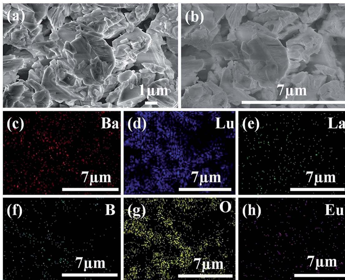
Fig. 2 (a) SEM micrograph of  $\text{Ba}_2\text{Lu}_{4.48}\text{Eu}_{0.5}\text{La}_{0.02}\text{B}_5\text{O}_{17}$  phosphors. (b–h) Elemental mapping profiles of  $\text{Ba}_2\text{Lu}_{4.48}\text{Eu}_{0.5}\text{La}_{0.02}\text{B}_5\text{O}_{17}$  phosphors.
