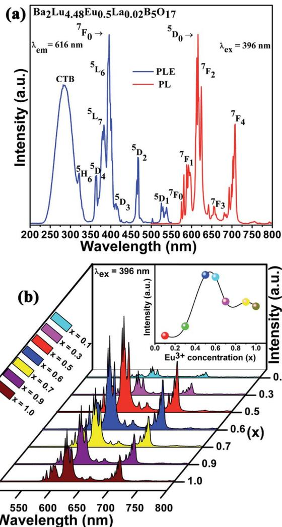
Fig. 3 (a) PLE ( $\lambda_{em} = 616$  nm) and PL ( $\lambda_{ex} = 396$  nm) spectra of  $Ba_2Lu_{4.48}Eu_{0.5}La_{0.02}B_5O_{17}$ ; (b) PL spectra for  $Ba_2Lu_{4.98-x}Eu_xLa_{0.02}B_5O_{17}$  ( $x = 0.1, 0.3, 0.5, 0.6, 0.7, 0.9$  and  $1.0$ ) phosphors. Inset shows the PL intensity as a function of  $Eu^{3+}$  concentration.
