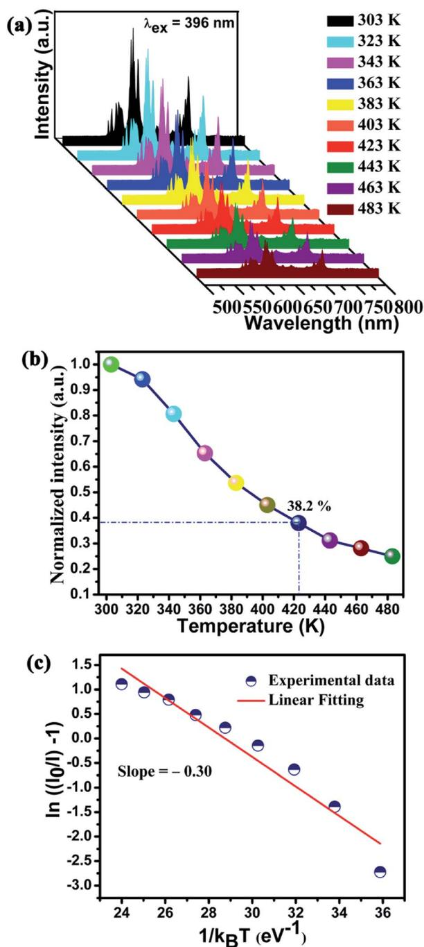
Fig. 7 (a) PL spectra of  $\text{Ba}_2\text{Lu}_{4.48}\text{Eu}_{0.5}\text{La}_{0.02}\text{B}_5\text{O}_{17}$  phosphors ( $\lambda_{\text{ex}} = 396 \text{ nm}$ ) with different temperature; (b) the normalized PL intensities as a function of the temperature; (c) relationship of  $\ln[(I_0/I) - 1]$  versus  $1/k_B T$  for  $\text{Ba}_2\text{Lu}_{4.48}\text{Eu}_{0.5}\text{La}_{0.02}\text{B}_5\text{O}_{17}$  phosphors.
