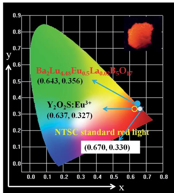
Fig. 6 CIE chromaticity diagram for  $\text{Ba}_2\text{Lu}_{4.48}\text{Eu}_{0.5}\text{La}_{0.02}\text{B}_5\text{O}_{17}$  red phosphors. Inset shows the digital photograph of optimal  $\text{Ba}_2\text{Lu}_{4.48}\text{Eu}_{0.5}\text{La}_{0.02}\text{B}_5\text{O}_{17}$  phosphors under 365 nm UV lamp.
