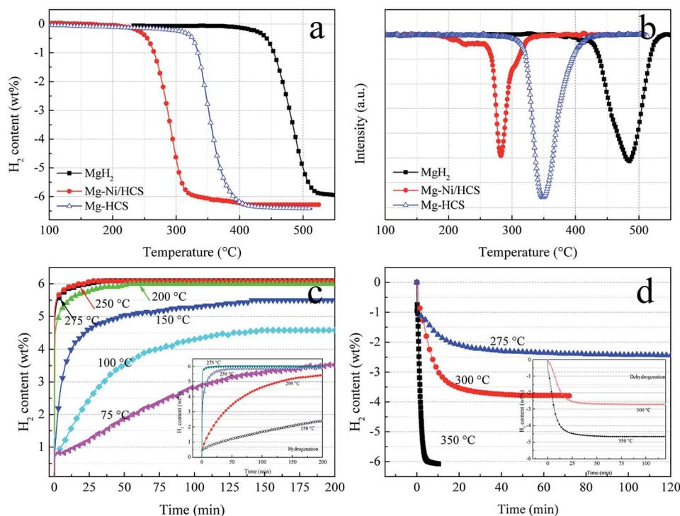
Fig. 7 TPD curves (a) and (b) of pure  $\text{MgH}_2$ , Mg–HCS, and Mg–Ni/HCS composites. Hydrogenation (c) and dehydrogenation (d) curves of Mg–Ni/HCS composite at various temperatures. The insets of (c) and (d) show the hydrogenation and dehydrogenation curves of Mg–HCS composite at various temperatures, respectively.
