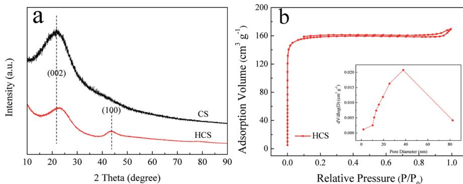
Fig. 1 X-ray diffraction (XRD) profiles (a) of the obtained CS and HCS; N<sub>2</sub> adsorption–desorption isotherms and the corresponding pore size distribution curves (b) of HCS.
