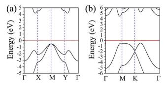
Fig. 5 Electronic band structures of (a)  $\alpha-BeH_2$  and (b)  $\beta-BeH_2$  monolayers at the PBE level.
