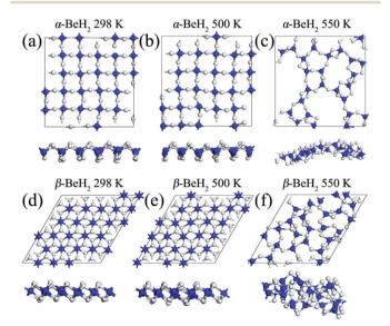
Fig. 3 Top (upper) and side (bottom) views of geometric configuration of  $\alpha\text{-BeH}_2$  and  $\beta\text{-BeH}_2$  monolayers after 20 ps AIMD simulations at (a and d) 298 K, (b and e) 500 K and (c and f) 550 K, respectively. Big blue balls represent Be atoms, and small white balls represent H atoms.
