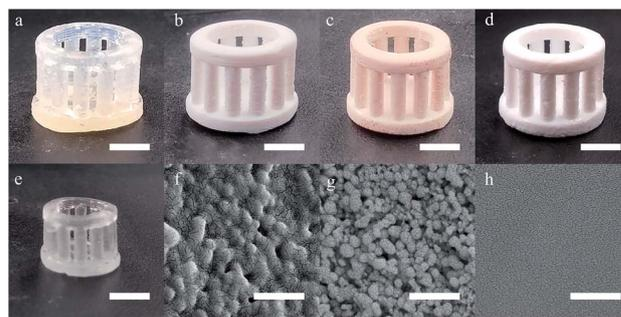
Fig. 6 (a–e) Photographs of the samples after heat treatments at room temperature, 150  $^{\circ}\text{C}$ , 250  $^{\circ}\text{C}$ , 500  $^{\circ}\text{C}$  and 1250  $^{\circ}\text{C}$  (scale bar, 5 mm). (f–h) SEM images of the samples after heat treatments at room temperature, 500  $^{\circ}\text{C}$  and 1250  $^{\circ}\text{C}$  (scale bar, 500 nm).
