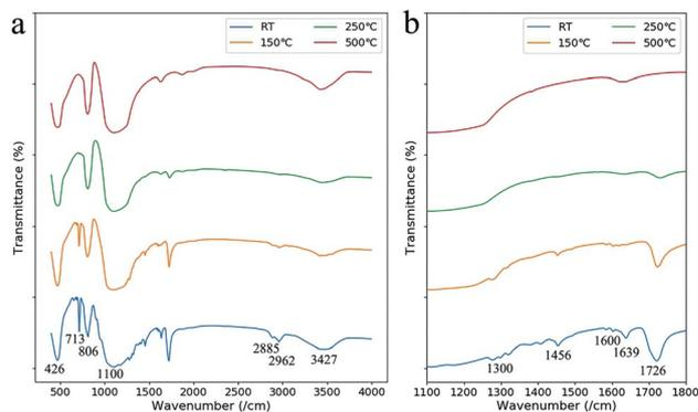
Fig. 5 (a) IR absorption spectra of the green parts after heat treatments at different temperatures (room temperature (RT), 150  $^{\circ}\text{C}$ , 250  $^{\circ}\text{C}$ , and 500  $^{\circ}\text{C}$ ). (b) The IR absorption spectra in the range of 1100–1800  $\text{cm}^{-1}$ .
