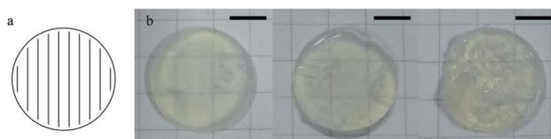
Fig. 3 (a) Illustration of the scan path for a cycloidal pattern (the red line represents the hatch distance), (b) photos of the green parts (cylinder with diameters of 14 mm and thicknesses of 1.4 mm) fabricated under different SL parameters (from left to right, 60 mW 46  $\text{mm s}^{-1}$ , 130 mW 100  $\text{mm s}^{-1}$  and 200 mW 154  $\text{mm s}^{-1}$ , scale bar, 2.5 mm).
