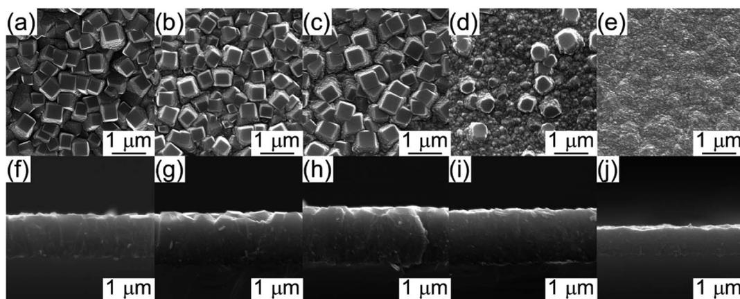
Fig. 2 Surficial and cross-sectional SEM image of diamond films deposited at  $T_{\text{sub}} = 1073$  K and various  $\text{CH}_4/\text{H}_2$  ratio ( $\eta_{\text{c}}$ ): (a and f) 0.5, (b and g) 1.0, (c and h) 1.5, (d and i) 2.0 and (e and j) 2.5 vol%.
