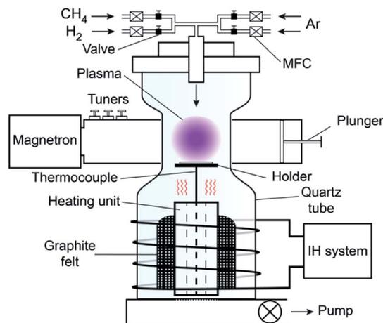
Fig. 1 Schematic diagram of the IH-MPCVD system.
