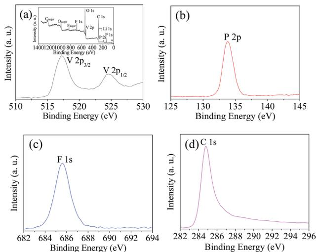
Fig. 7 XPS of V 2p (a), P 2p (b), F 1s (c) and C 1s (d) in sample LVPF800.
