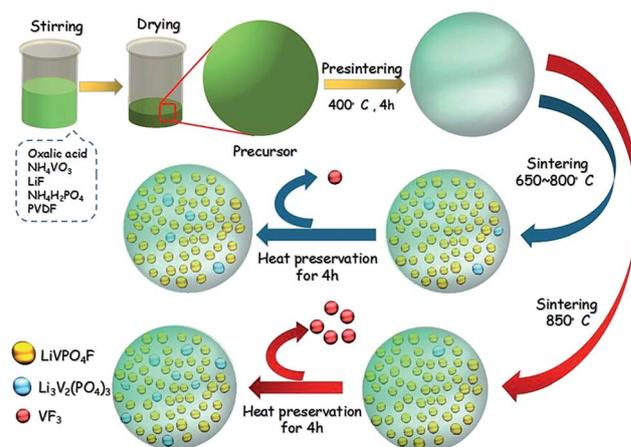
Scheme 1 Scheme of the fabrication process for  $\text{LiVPO}_4\text{F}$ .
