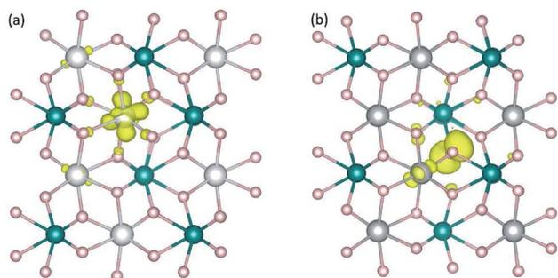
Fig. 3 Charge densities associated with hole polaron (a) η<sub>Co</sub><sup>+</sup> in CoWO<sub>4</sub> and (b) η<sub>O</sub><sup>+</sup> in NiWO<sub>4</sub>. The isovalue for the isosurface (yellow) is set to 0.05 e/Å<sup>3</sup>. Large (gray) spheres are Co or Ni, medium (blue) spheres are W, and small (red) spheres are O.
