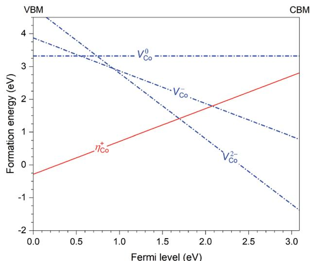
Fig. 4 Formation energies of the hole polaron ( $\eta_{\text{Co}}^+$ ) and Co vacancies ( $V_{\text{Co}}$ ) in  $\text{CoWO}_4$ , plotted as a function of Fermi level from the valence-band maximum (VBM) to the conduction-band minimum (CBM).
