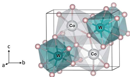
Fig. 1 Crystal structure of monoclinic  $CoWO_4$ . Large (gray) spheres are Co, medium (blue) spheres are W, and small (red) spheres are O.
