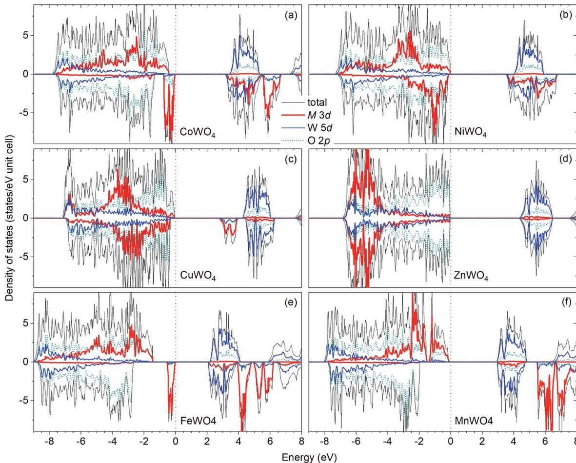
Fig. 2 Total and projected electronic density of states of  $MWO_4$  in the ferromagnetic spin configuration: (a)  $M = \text{Co}$ , (b)  $M = \text{Ni}$ , (c)  $M = \text{Cu}$ , and (d)  $M = \text{Zn}$ . The results for (e)  $\text{FeWO}_4$  and (f)  $\text{MnWO}_4$  are also included for comparison. The zero of energy is set to the highest occupied states.
