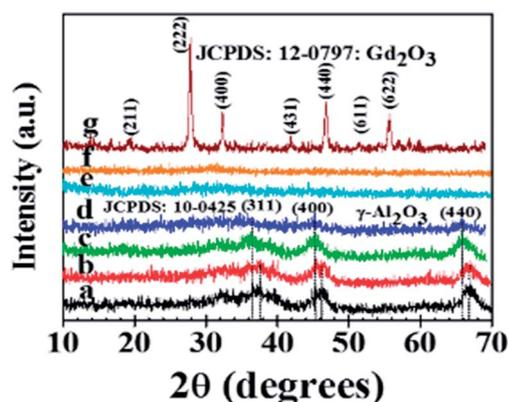
**Fig. 2** X-ray diffraction patterns of the Ag/Al–Gd-*x* photocatalysts: (a) Ag/Al<sub>2</sub>O<sub>3</sub>; (b) Ag/Al–Gd-2; (c) Ag/Al–Gd-5; (d) Ag/Al–Gd-15; (e) Ag/Al–Gd-25; (f) Ag/Al–Gd-50; (g) Ag/Gd<sub>2</sub>O<sub>3</sub>.
