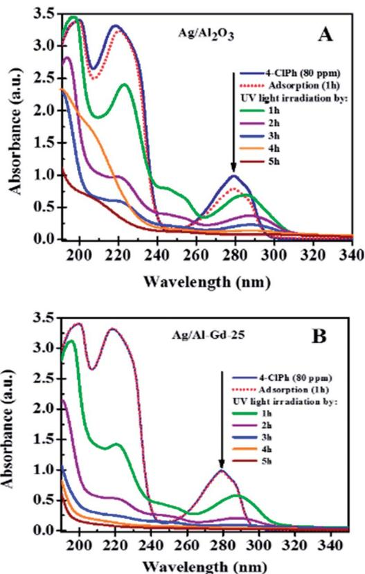
Fig. 10 UV-Vis spectra of 4-chlorophenol after UV light irradiation by 5 h using: (A) Ag/Al<sub>2</sub>O<sub>3</sub> and (B) Ag/Al-Gd-25 photocatalysts.
