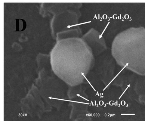
Fig. 5 SEM micrographs of Ag/Al-Gd-25 photocatalyst: (A)  $\times 11\,000$ ; (B)  $\times 11\,000$ ; (C)  $\times 37\,000$ ; (D)  $\times 60\,000$ .
