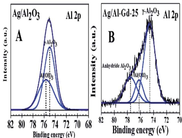
Fig. 8 XPS spectra of Al 2p for: (A) Ag/Al<sub>2</sub>O<sub>3</sub>; (B) Ag/Al-Gd-25.
