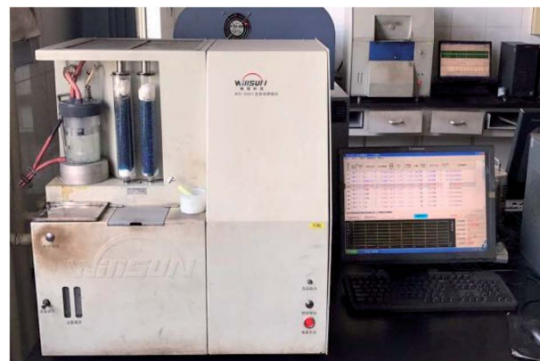
Fig. 4 The automatic sulfur meter (WS-S501).
