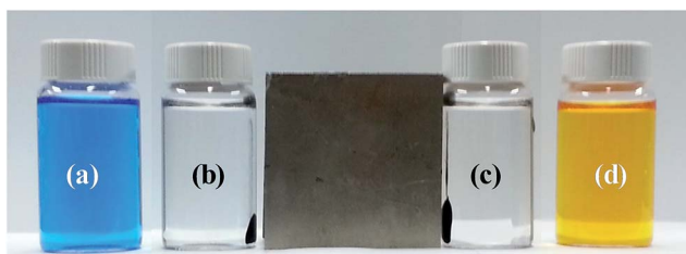
Fig. 6 Photographs of aqueous solutions of (a) MB and (d) MO and the FeCo/GC NCs@MSNs-SH collected using a magnet in the aqueous solutions after the adsorption of the organic dyes, MB (b) and MO (c).
