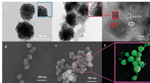
**Fig. 1** Characterization of as-synthesized NPs: (a) TEM and (d) SEM images of  $\text{Fe}_3\text{O}_4@CS$  nanoclusters. (b) TEM images, (e) SEM image and (f) elemental mapping of  $\text{Fe}_3\text{O}_4@CS/CuS$  NPs (copper (red) and iron (green)). (c) HRTEM image of  $\text{Fe}_3\text{O}_4@CS/CuS$  NPs.
