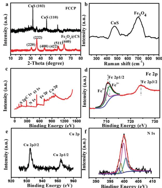
Fig. 2 (a) Powder XRD pattern, (b) Raman spectrum and (c) XPS survey spectrum of synthesized  $\text{Fe}_3\text{O}_4\text{@CS/CuS}$ . High-resolution XPS spectra of (d) Fe 2p, (e) Cu 2p and (f) N 1s of  $\text{Fe}_3\text{O}_4\text{@CS/CuS}$ .
