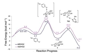
Fig. 2 Free energy profiles obtained using Umbrella Sampling simulations at the SCC-DFTB/ff03 level for the whole reaction in both DHQ2 enzymes [MtDHQ2 (blue), HpDHQ2 (magenta)]. For the 2<sup>nd</sup> step, free energies were corrected using single point MP2/6-31+G(d,p) calculations. For the 1st step in HpDHQ2 and the 3rd step in both enzymes, minimum free energy paths extracted from 2D free energy surfaces are shown.
