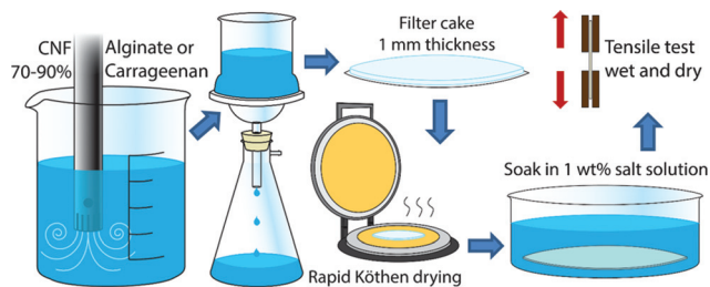
Fig. 1 Illustration showing the method of preparation of the nanopaper composites including: a mixing step, a filtration step, a drying step, and a post-treatment step with different ions by soaking the dried film.
