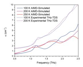
Fig. 6 AIMD-simulated IR spectra of  $\alpha$ -PCB at 100, 200, and 250 K (blue, purple, and red, respectively). The spectra exhibit a significant red-shift and spectral broadening as the temperature is increased.
