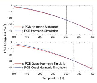
Fig. 7 Harmonic (top) and quasi-harmonic (bottom) free energy curves for the  $\alpha$ - and  $\gamma$ -PCB crystals (red and blue, respectively). The vertical dotted line is drawn at the intersection of the two curves, occurring at 301 K and 326 K for the harmonic and quasi-harmonic simulations, respectively. In both charts the data have been offset relative to the value of the  $\alpha$ -form free energy at 50 K.
