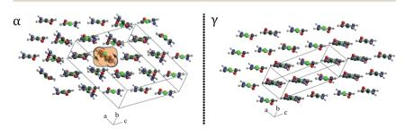
Fig. 3 Bulk static structures of the two forms of PCB, the low-temperature ordered  $\alpha$ -form (left) and the high-temperature plastic  $\gamma$ -crystal (right). The main structural difference between the two crystals is highlighted in orange, along with arrows denoting the hindered-rotational motion that drives the transformation between the two forms and corresponds to the vibrations discussed later in the text.
