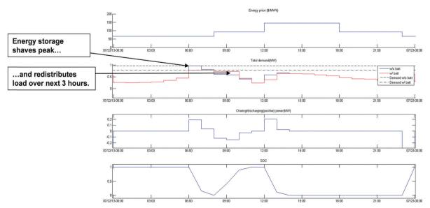
Fig. 3 Base load and battery operation for an illustrative day
