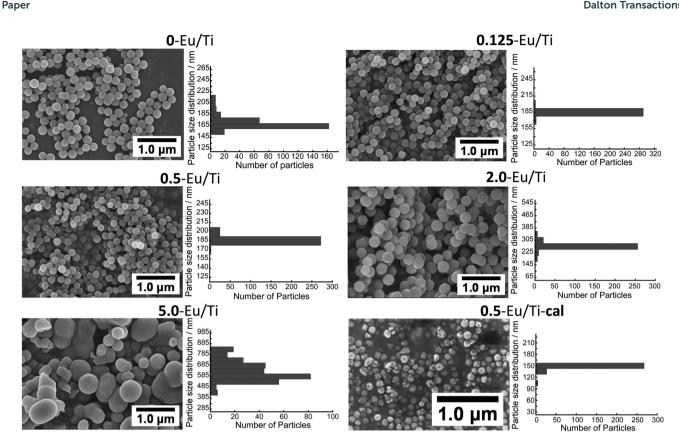
Fig. 2 FE-SEM images and the particle size distributions of Eu(acac)<sub>χ</sub>-doped titania particles with different Eu/Ti ratios. The D and CV values of the hybrids are summarized in Table 2.
