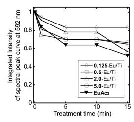
Fig. 7 Changes in the integrated intensity of the spectral peak curve at 592 nm of Eu(acac)<sub>3</sub> and Eu(acac)<sub>3</sub>-doped titania particles with different Eu/Ti ratios under the UV/ozone treatment for 15 min.
