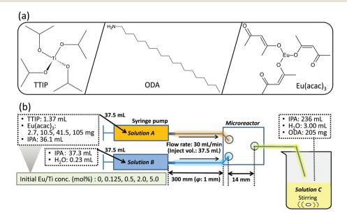
Scheme 1 (a) Chemical structures of the reagents used in this study and (b) an illustration of the experimental setup for the present microfluidic synthesis.
