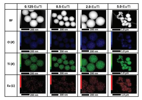
Fig. 3 STEM and EDX elemental mapping images of O, Ti and Eu atoms of Eu(acac)<sub>3</sub>-doped titania particles with different Eu/Ti ratios. STEM observation and elemental mapping were conducted at the same position.
