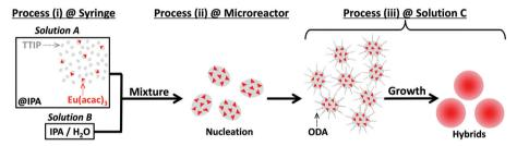
Scheme 2 Illustration for the proposed formation mechanism of Eu(acac)<sub>3</sub>-doped titania particles
