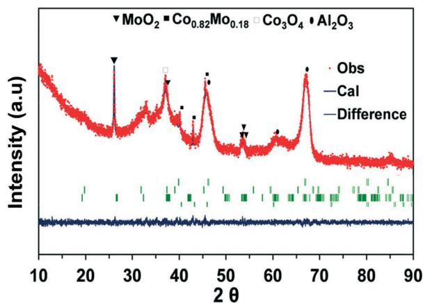
Fig. 6 XRD patterns fitted using the Rietveld refinement method for the CoMo<sub>2</sub> catalyst sample.  $\chi^2 = 1.12$ .
