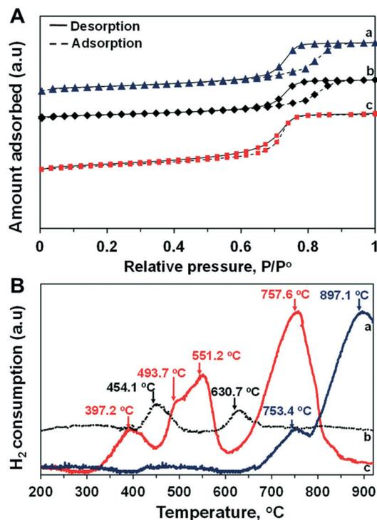
Fig. 4 N<sub>2</sub> adsorption/desorption isotherm curves (A) and TPR-H<sub>2</sub> profiles (B) of (a) Mo/Al<sub>2</sub>O<sub>3</sub>, (b) Co/Al<sub>2</sub>O<sub>3</sub>, and (c) CoMo<sub>2</sub> catalyst.
