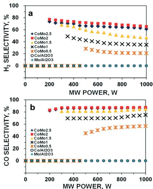
Fig. 2  $\text{H}_2$  selectivity (a) and  $\text{CO}$  selectivity (b) of DRM reaction for all the catalysts over MW irradiation at different MW power levels. Reaction parameters:  $\text{CH}_4/\text{CO}_2 = 1$ , VHSV =  $10 \text{ L g}^{-1} \text{ h}^{-1}$ .
