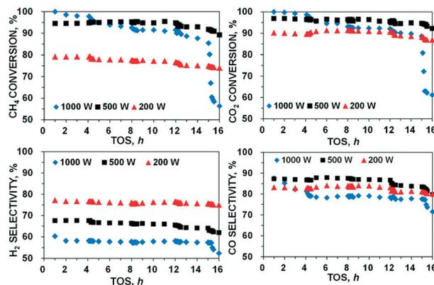
Fig. 3 Catalytic stability of CoMo<sub>2</sub> catalyst at three different MW power levels. Reaction parameters: CH<sub>4</sub>:CO<sub>2</sub> = 1, VHSV = 10 L g<sup>-1</sup> h<sup>-1</sup>.
