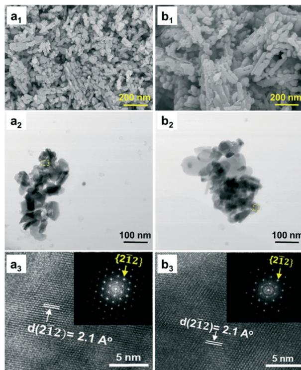
Fig. 7 FESEM (a<sub>1</sub> and b<sub>1</sub>), BF-STEM (a<sub>2</sub> and b<sub>2</sub>), and HRTEM images (a<sub>3</sub> and b<sub>3</sub>) of fresh (a<sub>1</sub>–a<sub>3</sub>) and spent (b<sub>1</sub>–b<sub>3</sub>) CoMo<sub>2</sub> catalysts. Reaction parameters: 200 W, CH<sub>4</sub>:CO<sub>2</sub> = 1, VHSV = 10 L g<sup>-1</sup> h<sup>-1</sup>.
