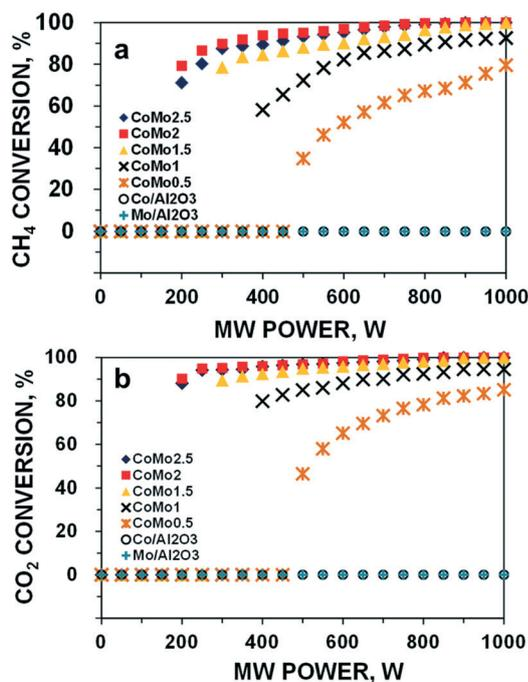
Fig. 1  $\text{CH}_4$  conversion (a) and  $\text{CO}_2$  conversions (b) of DRM reaction for all the catalysts over MW irradiation at different MW power levels. Reaction parameters:  $\text{CH}_4/\text{CO}_2 = 1$ , VHSV =  $10 \text{ L g}^{-1} \text{ h}^{-1}$ .
