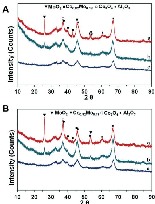
Fig. 5 XRD of fresh (A) and spent (B) catalysts: (a) CoMo<sub>2</sub>; (b) Mo/Al<sub>2</sub>O<sub>3</sub>; (c) Co/Al<sub>2</sub>O<sub>3</sub>. Reaction parameters: 500 W, CH<sub>4</sub>:CO<sub>2</sub> = 1, VHSV = 10 L g<sup>-1</sup> h<sup>-1</sup>.
