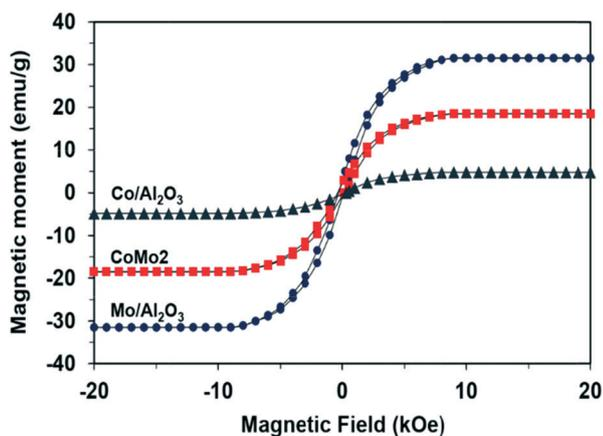
Fig. 9 Hysteresis loops of the curves of fresh Mo/Al<sub>2</sub>O<sub>3</sub>, Co/Al<sub>2</sub>O<sub>3</sub>, and CoMo<sub>2</sub> catalysts.
