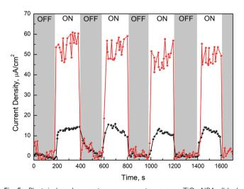
Fig. 5 Photoinduced current measurements on pure TiO2 NRAs (black line) and multisegmented Au/TiO2 NRAs (red line) with and without light
