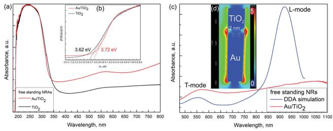
Fig. 3 (a) UV-Vis DR spectra of pure TiO2 and Au/TiO2 NRAs (b) Tauc plot analysis for band gap width. (c) Comparison between UV-Vis DR spectra of Au/TiO<sub>2</sub> and DDA simulation on Au NR. (d) Enhancement in electric field intensity for a multisegmented Au/TiO<sub>2</sub> NR.
