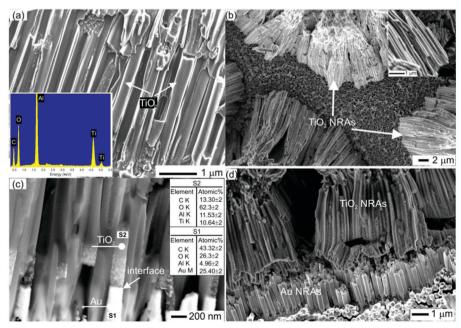
Fig. 1 (a) SEM image of the TiO<sub>2</sub> NRAs embedded inside the AAO membrane, inset shows SEM-EDS results of TiO<sub>2</sub> NRAs. (b) SEM image of the free standing TiO<sub>2</sub> NRAs after removing the AAO membrane (top view) (c) SEM image of the multisegmented (Au/TiO<sub>2</sub>) NRAs embedded inside the AAO membrane (inset shows SEM-EDS results of Au and TiO2 segments). (d) SEM image of the free standing multisegmented (Au/TiO2) NRAs.
