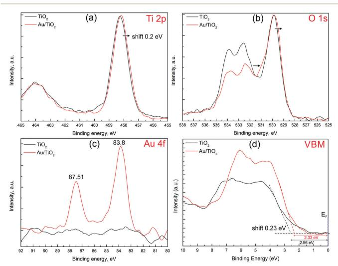
Fig. 4 XPS analysis of pure TiO<sub>2</sub> (black lines) and Au/TiO<sub>2</sub> (red lines): (a) Ti 2p, (b) O 1s, (c) Au 4f spectra and (d) determination of VBM.
