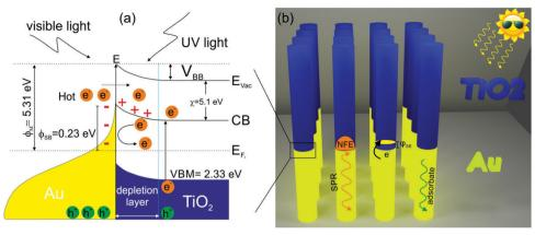
Fig. 6 (a) Band diagram of the Au/TiO<sub>2</sub> system, the optical process, hot electron injection, generation of SBH at the interface. (b) Schematic image of the free standing multisegmented (Au/TiO<sub>2</sub>) NRAs.
