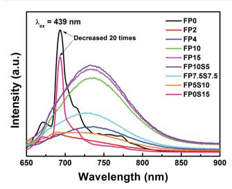
Fig. 5 PL spectra of FP and FPS glasses doped with 0.05 mol% Cr<sub>2</sub>O<sub>3</sub>.
