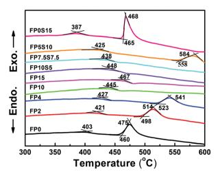
Fig. 3 Differential thermal analyses across the  $T_{\rm g}$  region of FP and FPS alasses and melts
