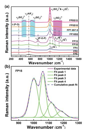
Fig. 4 (a) Raman spectra of the FP and FPS glasses and (b) example of Gaussian deconvolution on FP15 (see the text for assignment details).
