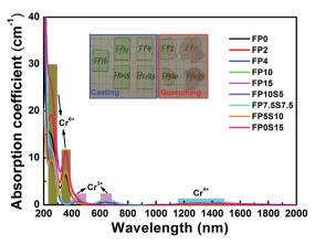
**Fig. 1** Optical absorption spectra of chromium-doped FP and FPS glasses. The inset shows sample photographs (mesh spacing of 5 mm).
