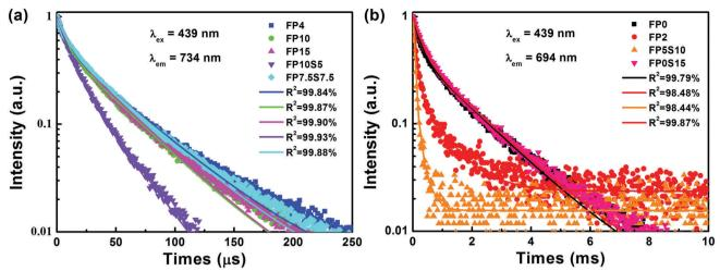
Fig. 7 Luminescence decay curves of Cr<sup>3+</sup>-doped (a) casting samples and (b) quenching samples.
