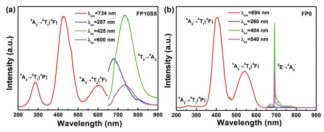
Fig. 6 PLE and PL spectra of selected (a) FP10S5 and (b) FP0 glasses doped with 0.05 mol% Cr<sub>2</sub>O<sub>3</sub>
