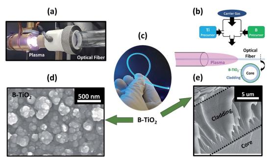
Fig. 1 (a) Photo of the microwave plasma reactor and PMMA optical fibre being coated while passing through the plasma; (b) simplified scheme of the plasma coating process; (c) photo of the illuminated PMMA optical fibres coated with B-TiO<sub>2</sub>; (d) SEM top view and (e) SEM cross-sectional images of the B-TiO<sub>2</sub> thin film deposited by AP-PECVD on the optical fibres.
