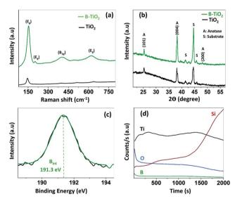
Fig. 2 (a) Raman spectra of the anatase B-TiO $_2$  thin film deposited on the polymeric optical fibre (POF). The Raman spectra of the undoped TiO $_2$  thin film on the POF are shown for comparison; (b) XRD patterns of the B-TiO $_2$  thin film deposited on planar silicon wafers; (c) XPS spectrum of the B 1s core level for the B-TiO $_2$  thin film on the POF and (d) D-SIMS spectra of the B-TiO $_2$  thin film on planar silicon wafers.
