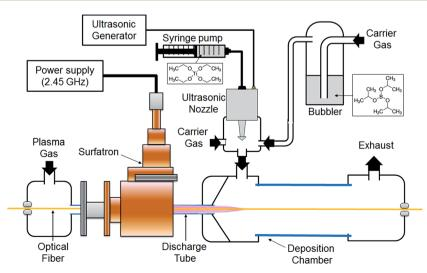
Fig. 4 Schematic of the AP-PECVD apparatus set up for doping.
