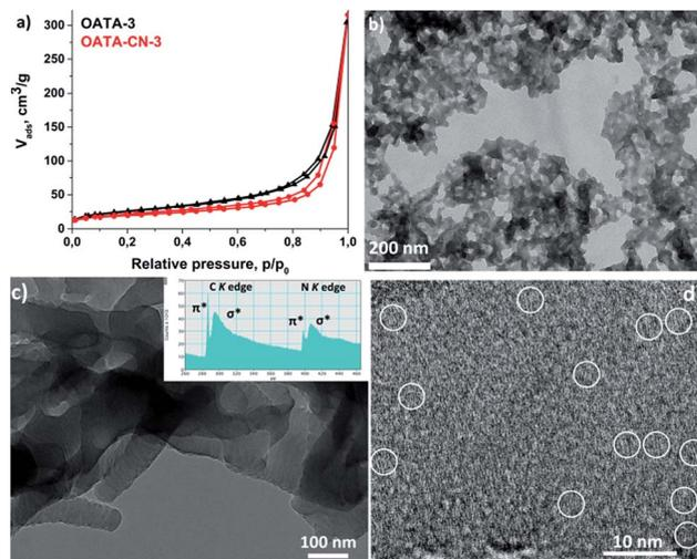
Fig. 5  $\text{N}_2$  sorption isotherms of OATA-3 and OATA-CN-3 (a); TEM image of OATA-CN-3 (b) and HR-TEM images of OATA-CN-2 (c and d). Inset in (c) shows the EEL spectrum of carbon and nitrogen K edges.
