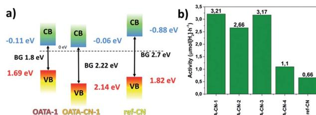
Fig. 7 A schematic representation of the band structures of OATA-1 and OATA-CN-1 (a); activity of OATA-CN-*N* and ref-CN in a Pt-assisted HER upon visible light irradiation, using TEOA as a sacrificial agent (b).
